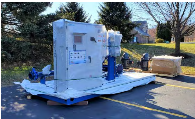
Soon to be installed 1000 GPM, Vertical Turbine Pump Station with 2- 60 hp pumps at Cobblestone Creek
